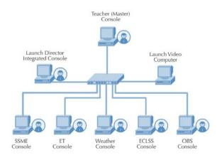
There are quite a few possibilities for setting up the simulation lab. There are 5 different KLASS student consoles. The SSME console is designed for 3 SSME engineers. In addition, the weather console has a primary view and 4 different views. There is also an integrated view that shows a summary of all systems. Ideally, an integrated simulation set-up could include these items:
